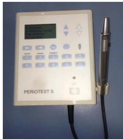
Figure 1. Apparatus for determining the mobility of teeth "PERIOTEST S" ("Siemens" Germany)
