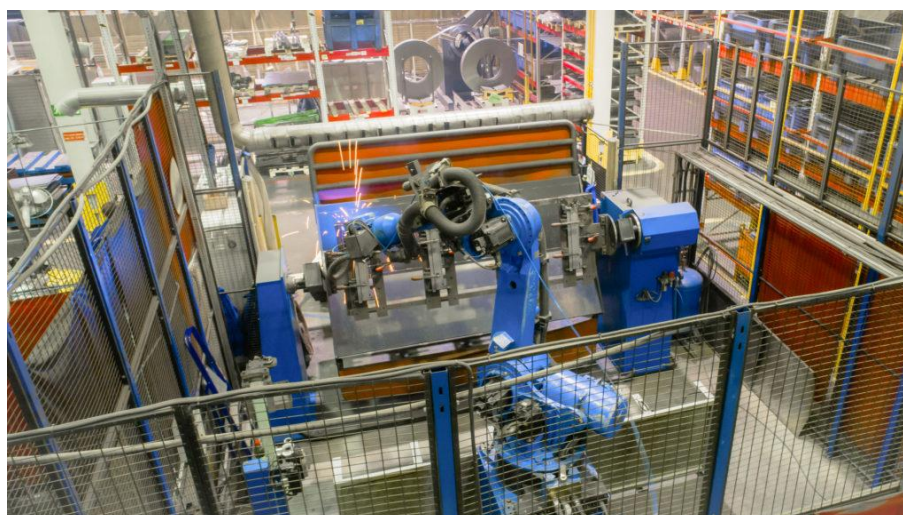
Figure 1. An traditional industrial robot requires a fence [2].
